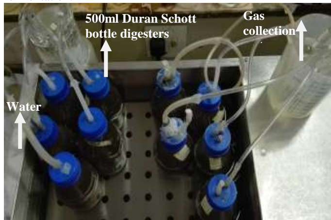
Fig 3: Picture showing the set-up of BMP test
