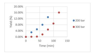
Fig. 2: Extraction yield versus pressure over time
