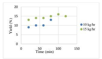
Fig. 3: Extraction yield versus solvent flowrate over time
