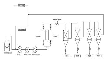
Fig. 1: Schematic for Supercritical Fluid pilot plant
