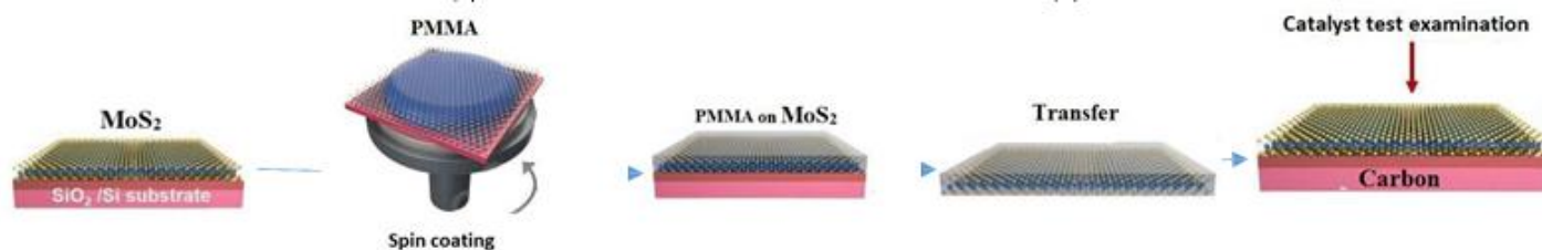
Fig. 1 .(a,b) plunge substrates in 0.1 M NaOH, and (c) transferring MoS 2 monolayer from SiO 2 to Carbon.
