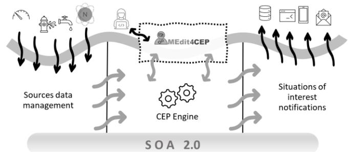
architecture and several additional tools, for the intelligent management of water supply networks. Although we will focus on the GEN group networks, it could be extended to other water supply networks or other IoT domains.
