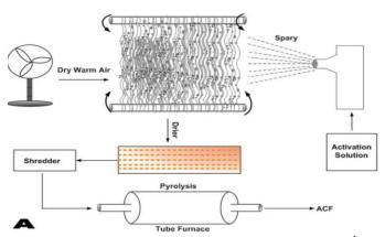
Fig. 2. Schematic representation of the preparation method for ACF using Agave Sisalana
