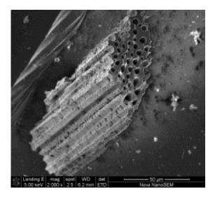
Fig. 3. SEM micrograph of sisal fibre after being pyrolysed by applying the activation reagents.
