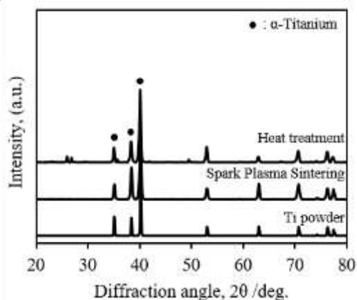
Fig. 2 XRD pattern of  $\text{Ti}+0\text{ZrO}_2$
