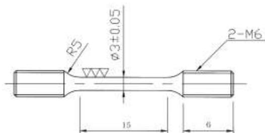
Fig. 1 Sketch of the tensile sample
