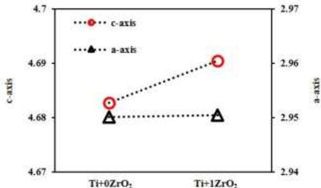
Fig. 5 Lattice constants of c-axis and a-axis of  $\text{Ti}+0\text{ZrO}_2$  and  $\text{Ti}+\text{ZrO}_2$  after hot extruded at  $850^\circ\text{C}$
