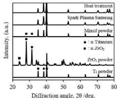
Fig. 3 XRD pattern of  $\text{Ti}+1\text{ZrO}_2$
