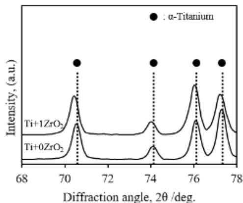
Fig. 4 Comparison of the XRD pattern of  $\text{Ti}+\text{ZrO}_2$  alloys
