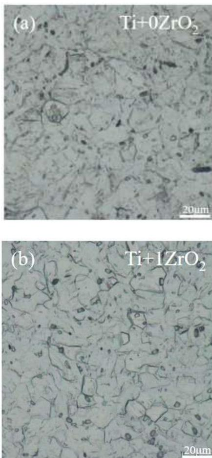
Fig. 6 Optical microstructures of (a) Ti+0ZrO<sub>2</sub>, hot extruded at 850°C, (b) Ti+1ZrO<sub>2</sub>, hot extruded at 850°C
