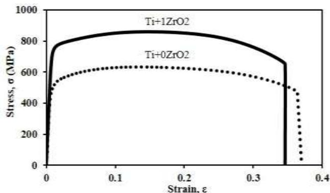
Fig. 7 Stress-strain curves of Ti+ZrO<sub>2</sub>, hot extruded at 850°C
