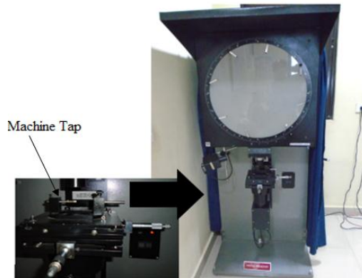
Fig.8. Machine Tap positioned in the Profile Projector for Wear measurement
