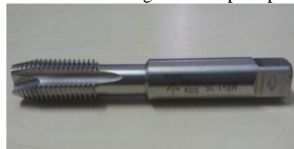
Fig.4. Photograph of HSS straight, three fluted spiral point tap, M8x1.25
