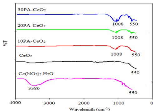
Fig. 3: FTIR result of cerium nitrate,  $\text{CeO}_2$  and  $\text{H}_3\text{PO}_4$ -modified  $\text{CeO}_2$  catalysts
