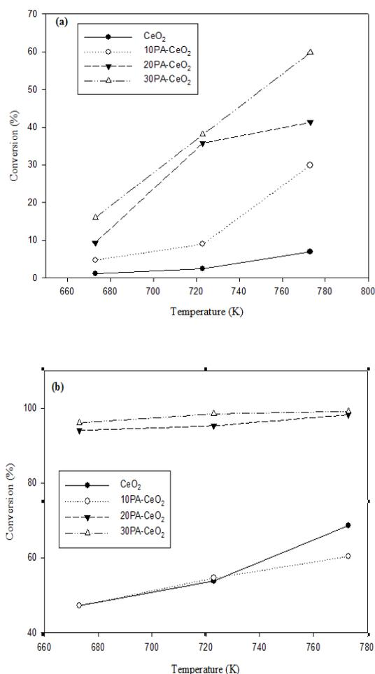
Fig. 4: Catalytic performance (a) ethanol conversion and (b) ethylene selectivity of  $\text{CeO}_2$  and  $\text{H}_3\text{PO}_4$ -modified  $\text{CeO}_2$  catalysts at 673 to 773K and ethanol partial pressure 33kPa.
