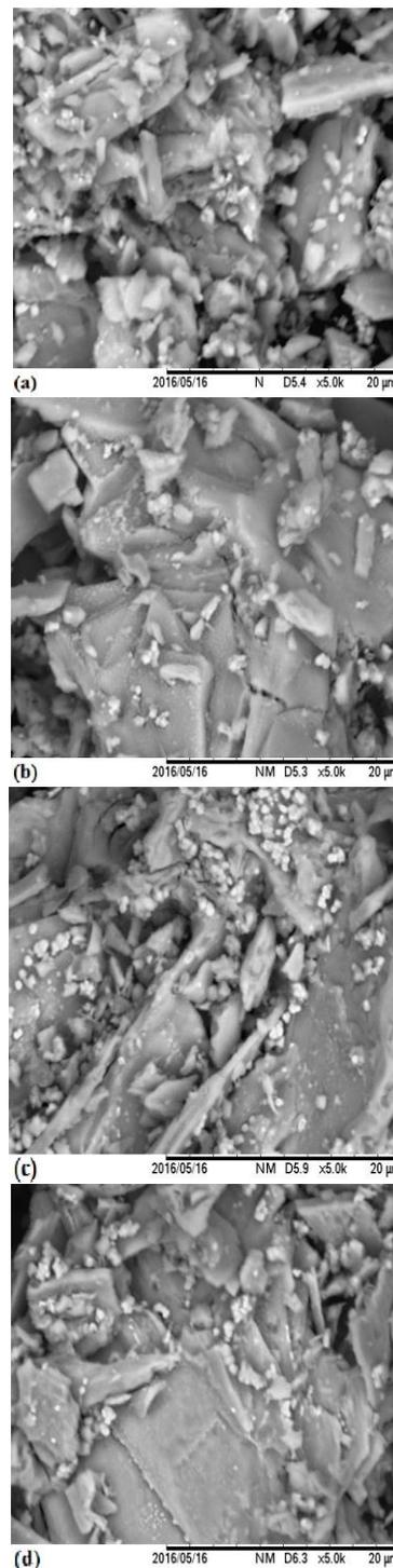
Fig. 2: SEM images of (a)  $\text{CeO}_2$ , (b) 10PA-  $\text{CeO}_2$ , (c) 20PA-  $\text{CeO}_2$  and (d) 30PA-  $\text{CeO}_2$  with magnification of 5K obtained from all fresh catalysts
