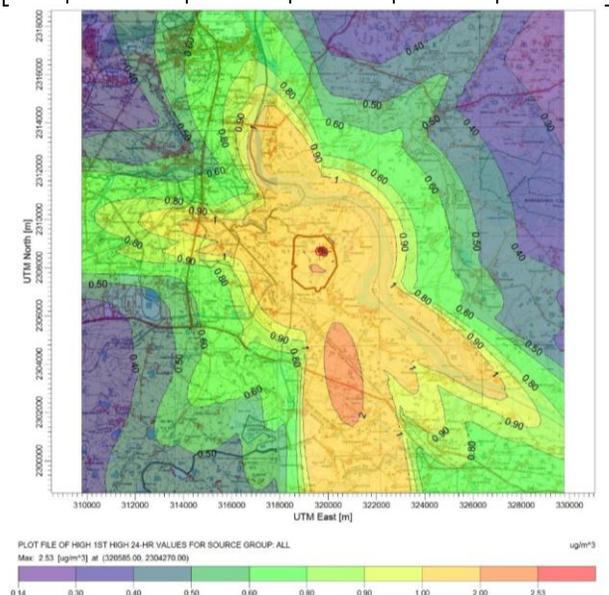
Fig. 2: Contour Plot of 24-Hour Maximum GLC's – Winter (PM10)
