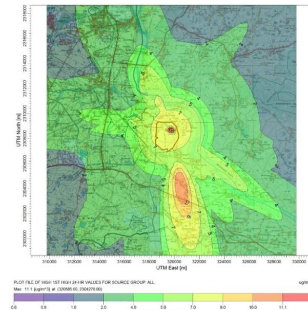
Fig. 3: Contour Plot of 24-Hour Maximum GLC's – Winter (NO<sub>x</sub>)
