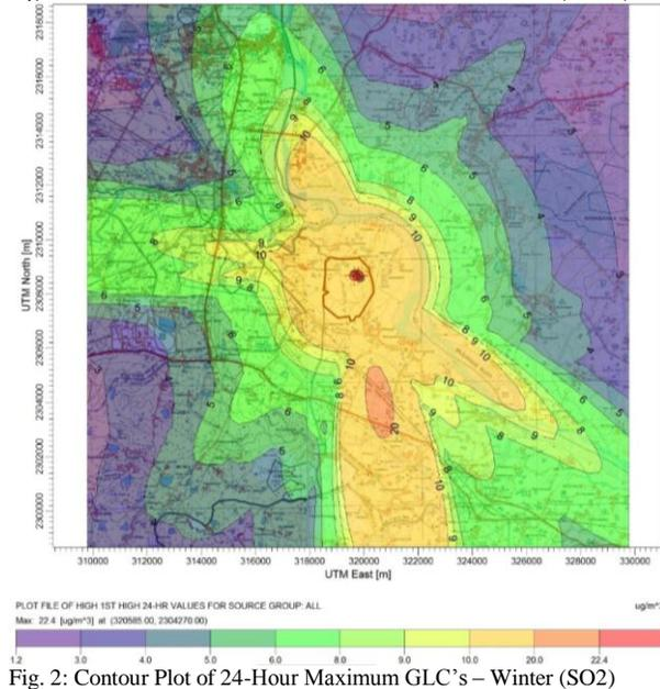
Fig. 2: Contour Plot of 24-Hour Maximum GLC's – Winter (SO<sub>2</sub>)
